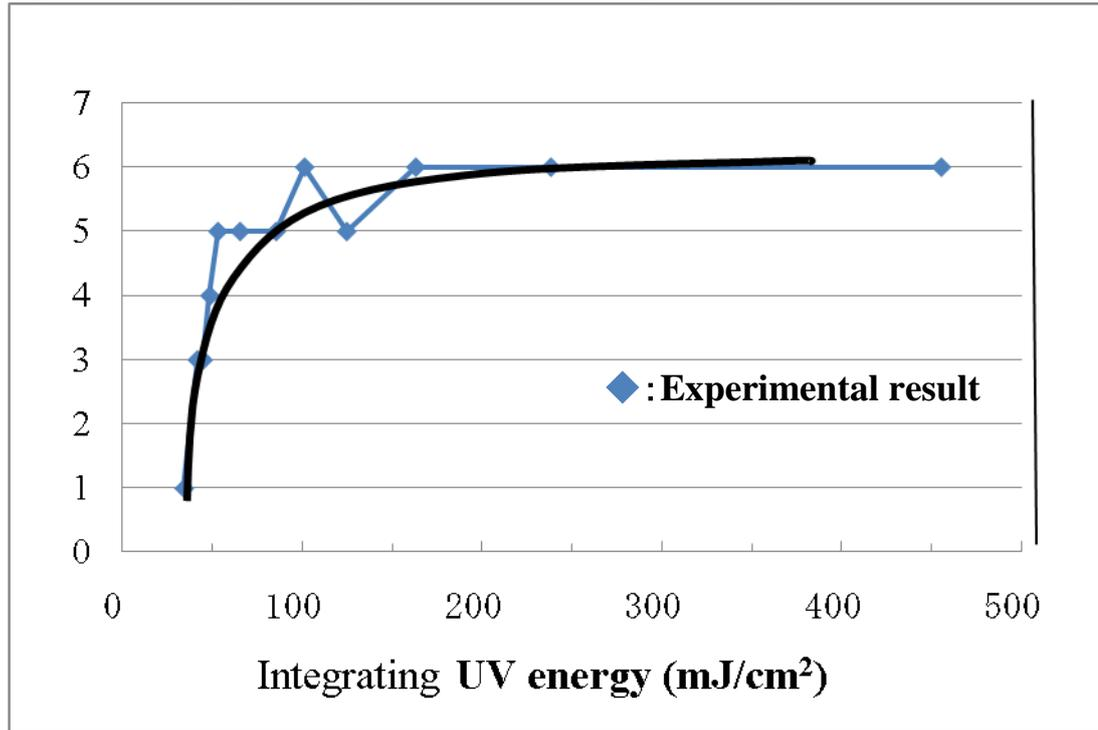
The hardening sensitivity was evaluated by a pencil hardness test. It was found that the ink could be completely cured by UV-LED light energy of about 150m J/cm2. The emission wavelength was 380nm. A sensitizer with about 350-390nm absorption capability was added to the ink.
